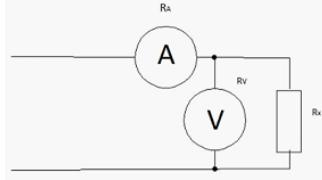
$$\text{a) } R_x = \frac{U}{I} \quad \text{б) } R_x = \frac{U}{I} - R_A \quad \text{в) } R_x = \frac{U}{I - \frac{U}{R_v}} \quad \text{г) } R_x = \frac{U}{I} - R_v - R_A$$
