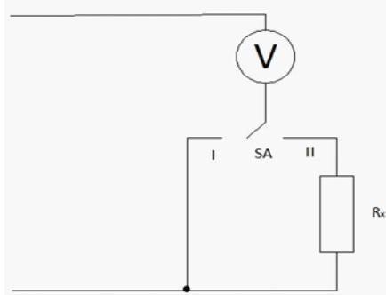
$$\text{а) } R_x = \frac{U_1}{U_2} R_v \quad \text{б) } R_x = \left( \frac{U_1 - U_2}{U_2} \right) R_v \quad \text{в) } R_x = \left( \frac{U_1}{U_2} + 1 \right) R_v \quad \text{г) } R_x = \left( \frac{U_2}{U_1} + 1 \right) R_v$$
