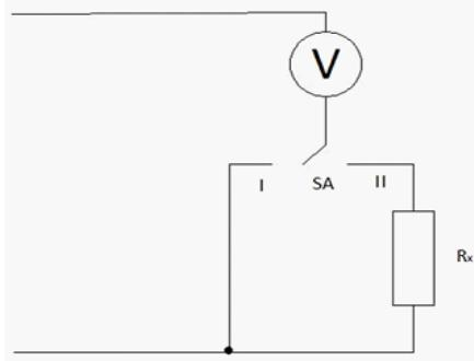
$$a) R_x = \frac{U_1}{U_2} R_v \quad 6) R_x = \left( \frac{U_1 - U_2}{U_2} \right) R_v \quad b) R_x = \left( \frac{U_1}{U_2} + 1 \right) R_v \quad \Gamma) R_x = \left( \frac{U_2}{U_1} + 1 \right) R_v$$
