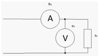
$$a) R_x = \frac{U}{I} \quad 6) R_x = \frac{U}{I} - R_A \quad b) R_x = \frac{U}{I - \frac{U}{R_v}} \quad \Gamma) R_x = \frac{U}{I} - R_v - R_A$$
